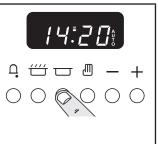
Set the oven to the required temperature. When your cooking is finished the beeper sounds. TURN THE OVEN KNOB TO 0 (off) FIRST, then press once to stop the beep, press again to return to manual cooking.
